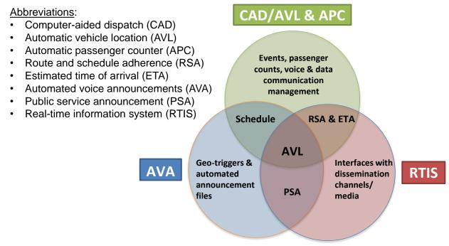
New Hampshire transit agencies that do not already have the core technologies shown in Figure 27 (most of Tier 1) should consider deployment of these specific technologies first, particularly CAD/AVL, which provides the backbone needed for the use of the other core technologies. Procuring the core technologies together can be less costly than purchasing them separately and having to integrate them. For example,
